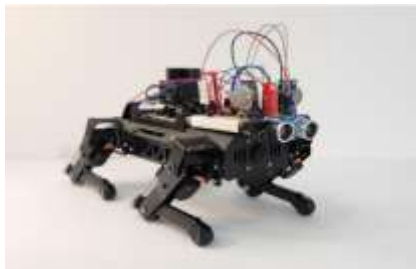
Figure 4 QRDs set up for structural inspection in confined spaces: a. Modified with multi-sensor module, and b. Teamed with microrobots that use vibratory locomotion and FPV cameras.
