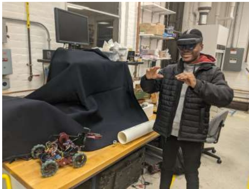
Figure 8 Use of augmented reality interface with first person view on microrobot to visualize conditions inside confined space.
