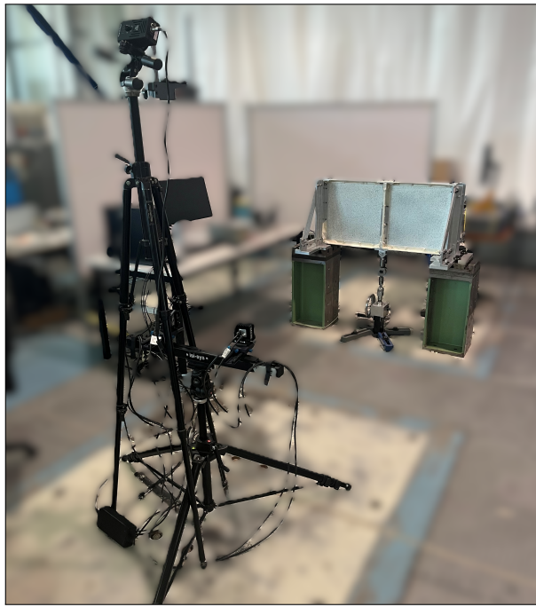
Figure 2. DIC measurement system with the speckled Wagner beam's panels.
