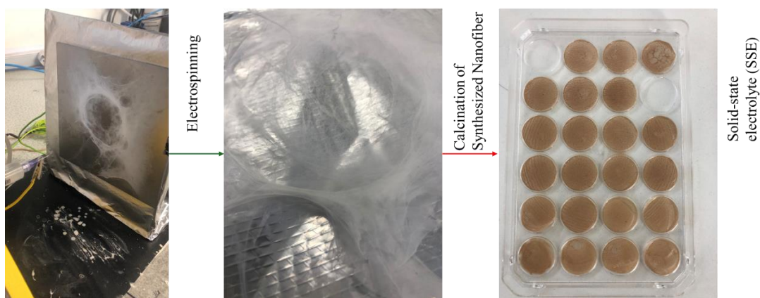
Figure 2: Step-by-step synthesis process for developing solid-state electrolyte.
