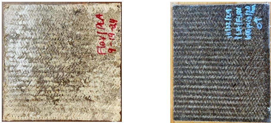
Figure 1. Photos of flax/PLA composites manufactured 9/19/2024 (left) and 10/22/2024 (right) using different manufacturing parameters. Composite A (left) is 15.24 cm x 15.24 cm and composite B (right) is 12.70 cm x 15.24 cm. Both samples are ~3-4 mm thick.
