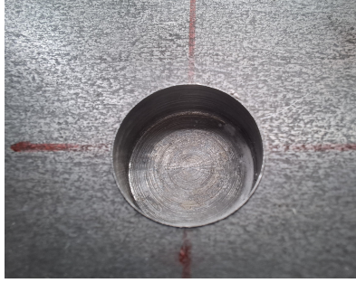
(a) artificial 4 mm depth defect (top view)
