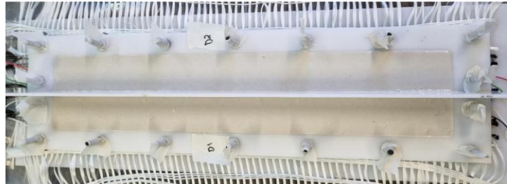
Figure 1. (a) Photo of the textile within the mold; (b) Carbon-based TRC specimens after casting.
