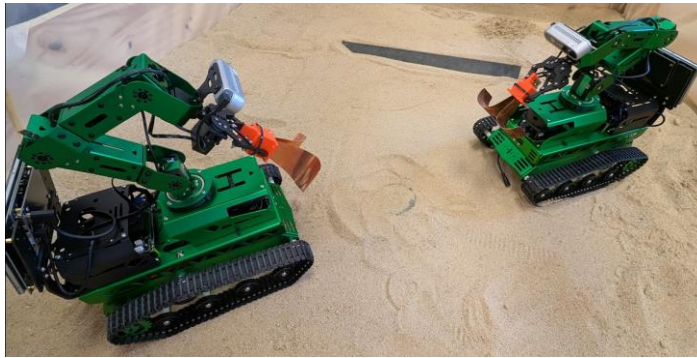
Figure 11 Mock-up of multi-static ground penetrating radar mounted on mobile robot with slant sensing capabilities.
