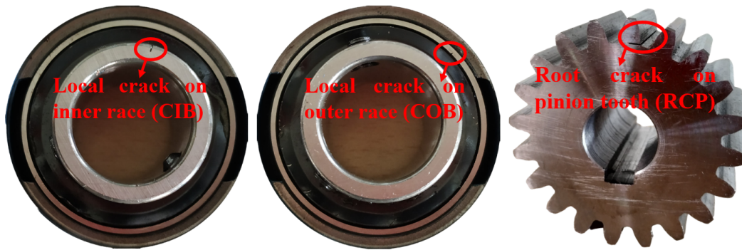
Figure 2. A glimpse of compound defects seeded – (left) Localized crack on bearing inner race, (middle) Localized crack on bearing outer race and (right) Localized root crack at pinion tooth.
